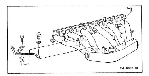
All parts bolted to removed intake manifold . . . . .
