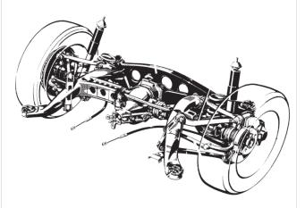
Enough for the theory and the objectives, let's look at the parts on the car. The rear suspensions of all current Mercedes-Benz cars share the same five-link geometry. The parts, to be sure, are not interchangeable between models, but the geometry is, as we learned in high school, congruent.
