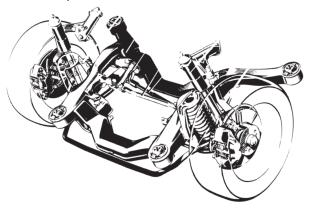
The current Mercedes-Benz front suspension looks simpler than the rear, though there are several variations. All share a lower wishbone with the damper strut as far outboard as is compatible with clearing the wheel and tire. The springs are as far inboard as possible to reduce their share of the unsprung weight. You make the alignment adjustments through eccentric inboard bushings and at the tierod ends. The swaybar extends across the front of the suspension.
