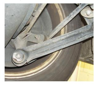
Running forward from the lowest part of the knuckle to the subframe, the pushing link transmits the drive forces from the knuckle forward to the body of the car. When the driver accelerates, the final, delivered engine torque applies to the vehicle mostly through the pushing link.
