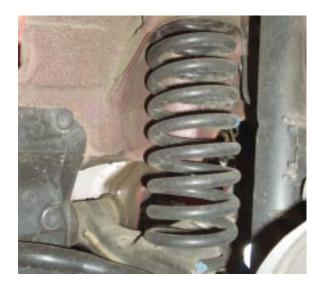
Certain models, beginning with the 140, use a small control arm at the top of the damper strut to better optimize caster and camber in certain driving modes. Some experienced mechanics find the angle of that small control arm is the quickest indication of any problem with suspension height, such as sagging springs. It pivots back as well as up in its normal travel, so once you've seen a few 'known-good's' one that's out of adjustment will leap out at you.
