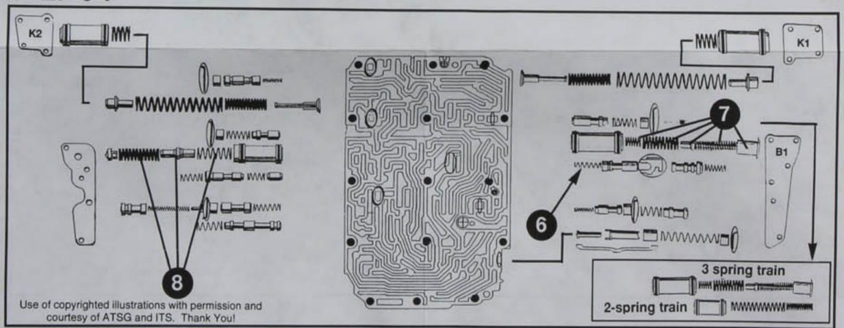
Total installation of this kit is essential for stabilization of shifts and the flexibility of fine adjustment by the modulator and TV cable
