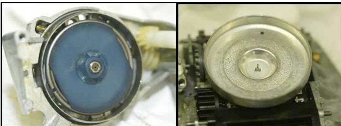
(Left) The pin from the top section fits delicately into the center of the blue section that links to the speedometer cable. As the cable turns the blue "disc", the pin also turns loosely, driving the needle.
