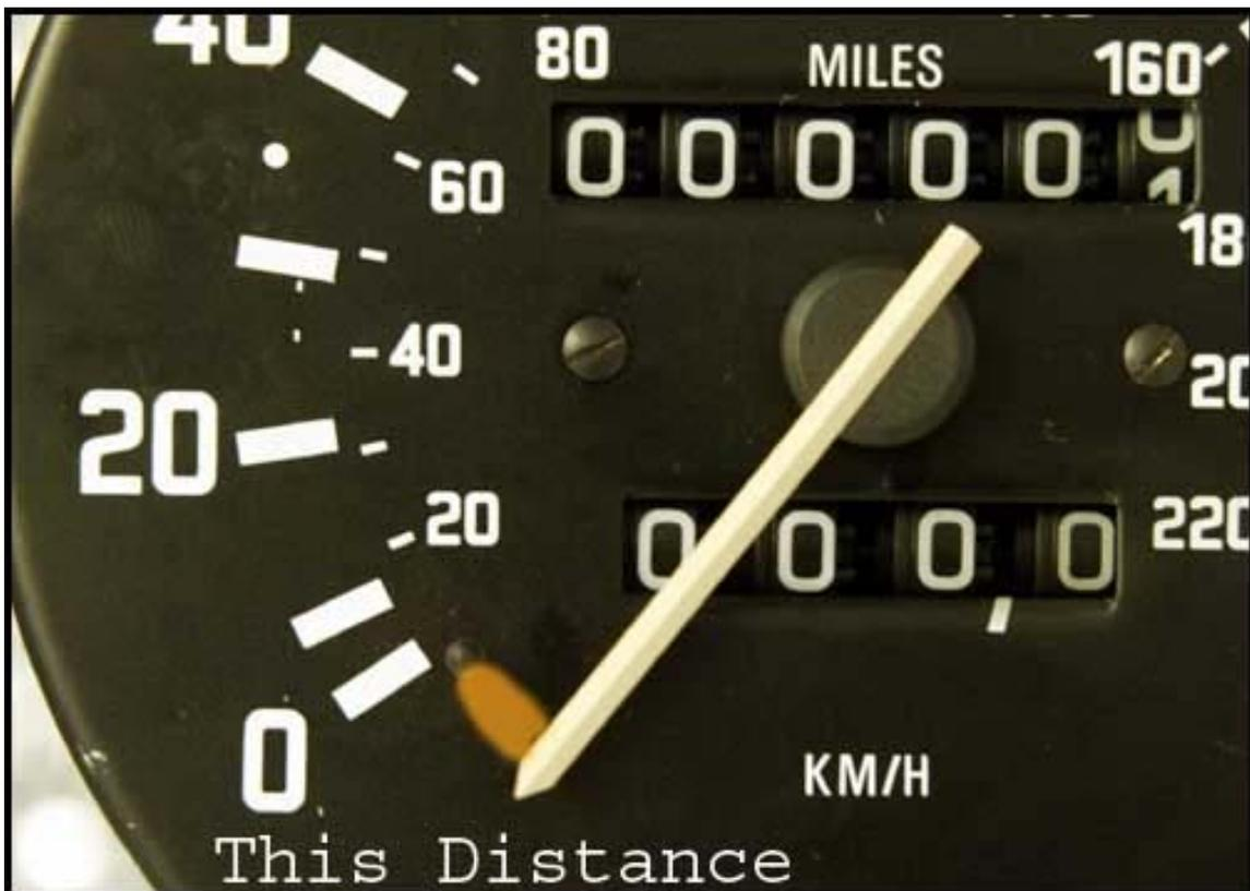
This is the part that I really am guessing about. When putting the needle back on, you need to pre-load the needle and then move it over the stop. The position of the needle in this photo was based on another speedometer that hasn't been taken apart. I would suggest a little trial and error to get the right position or stop by your local garage and get it recalibrated.
