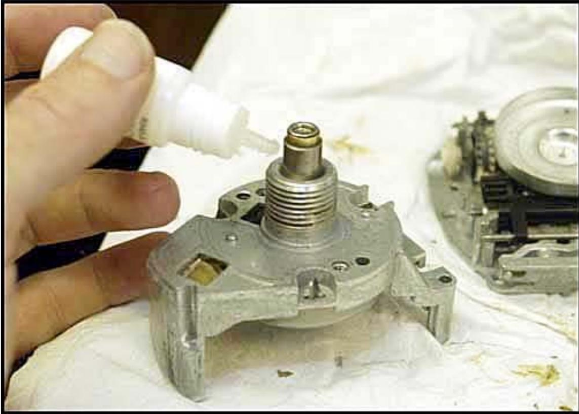
To reset the drive gear, I used common quickset glue. I carefully applied a few drops to the outside bearing and turned it in the housing until the glue gripped. Make sure you don't get any glue on the drive. The most critical part of this step is to set the drive gear to the correct height. This is why my speedometer was too stiff to begin with.
