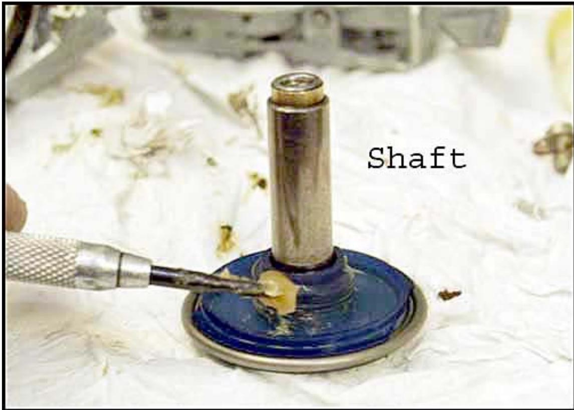
Using a small screwdriver, I re-applied axel grease to the drive gear, careful not to get it on the shaft.
