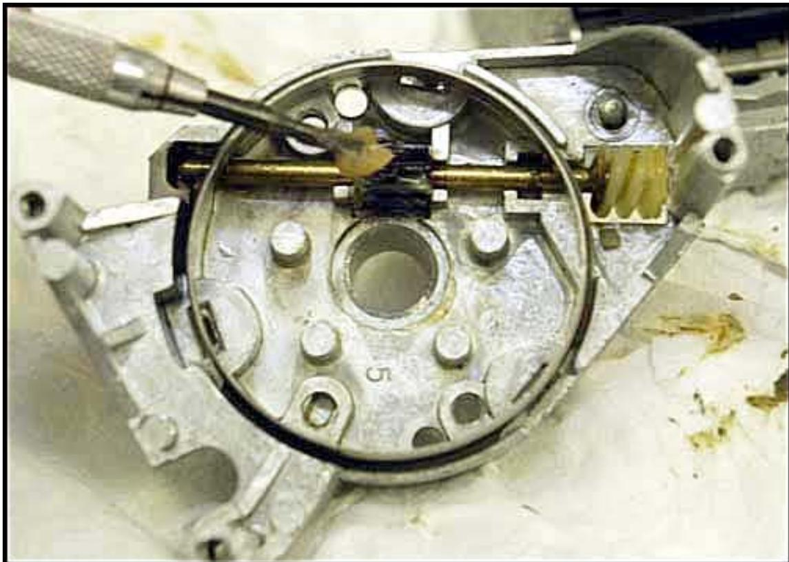
I washed out all the leftover glue and grease that worked it's way into the housing and re-applied grease to the gears. The ring holds down this shaft. If you want to remove it, use needle nose pliers to untwist the tabs. Otherwise, just use a paper towel and clean off the old grease before you re-apply the new grease.
