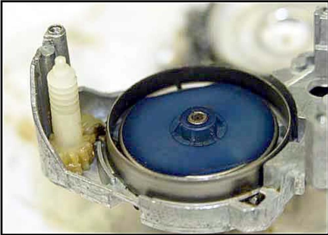
When putting the two halves back together, put the worm gear in first. Spin the drive a little until you feel the needle engage the drive gear. Put the three (3) screws back in and test spin the drive.
