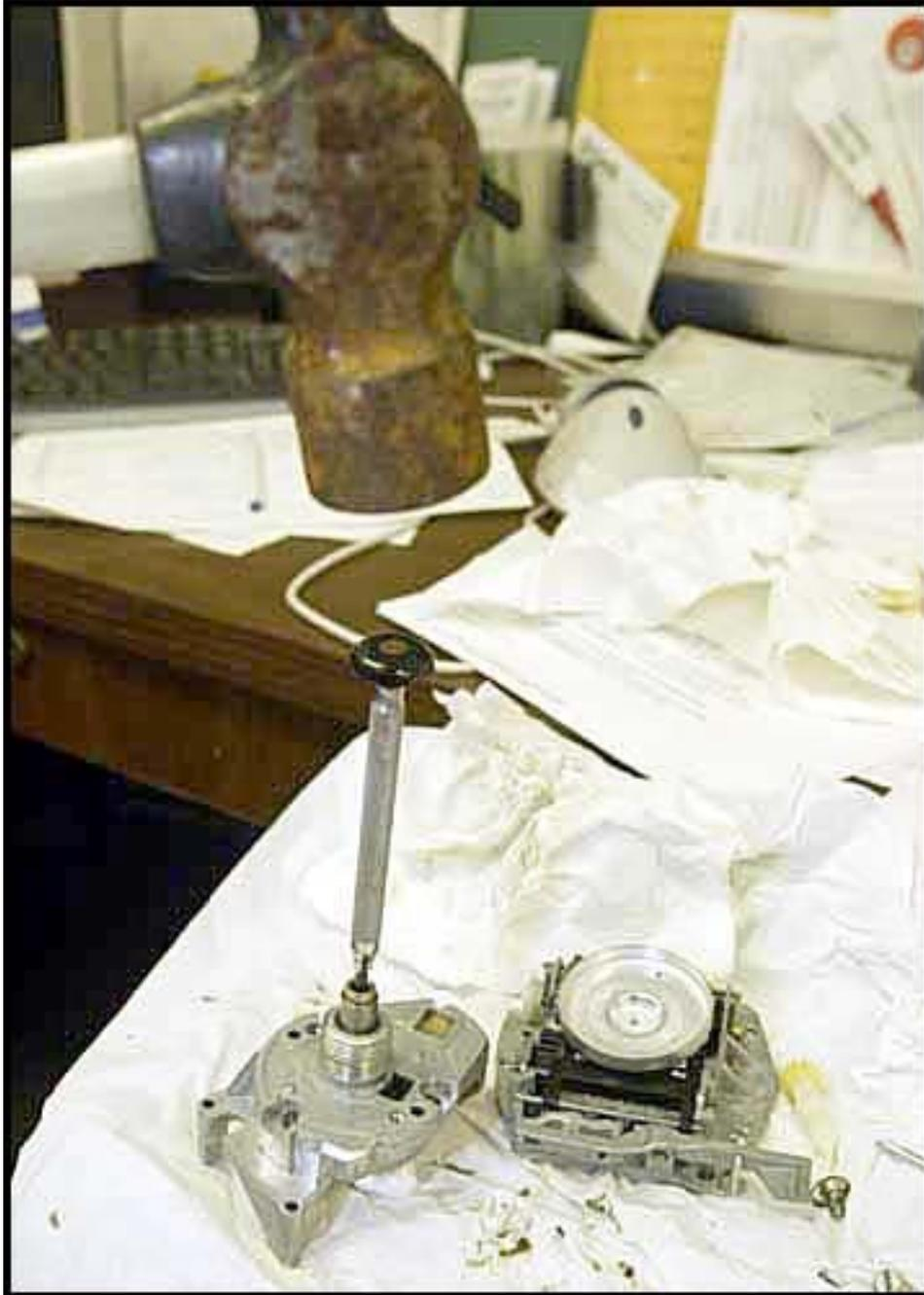
My speedometer was very stiff. I figured out the backside was knocked too far in and needed to be pulled back out. I also wanted to inspect the plastic gears while I had it apart. To do this, I knocked the drive gear out. It is held in by glue as far as I could tell.
