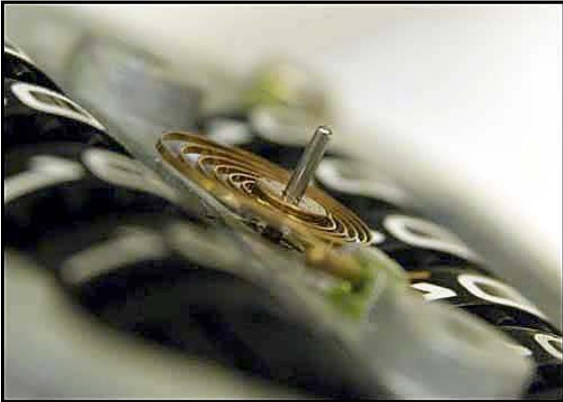
To figure out the proper position of the drive gear, when you reassemble the two halves, the needle spring should be level. If the center is low or high, the gears might not engage, the drive might be too stiff or the two halves won't fit together.
