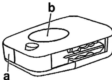
For 129's and 140's up to a build date of November 1993, point the transmitter window (a) toward an IR receiver and press the IR transmitter button (b). Then within 30 seconds, lock or unlock the vehicle using the mechanical key. Now the vehicle is synchronized to that transmitter.
