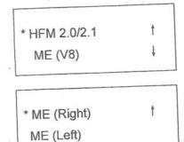
9. Press corresponding key to select ME type. For example, at the third screen display in step 8, press "\u2214" key to move the "\u221\*" symbol to point at "ME (Left)", then press "ENTER" key to select "ME (Left)", the screen displays:
