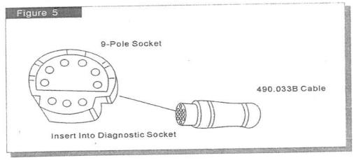
The 9-pole diagnostic socket comes with earlier model vehicles. It can display on-off ratio fault codes. Various on-off ratio meters are available.
