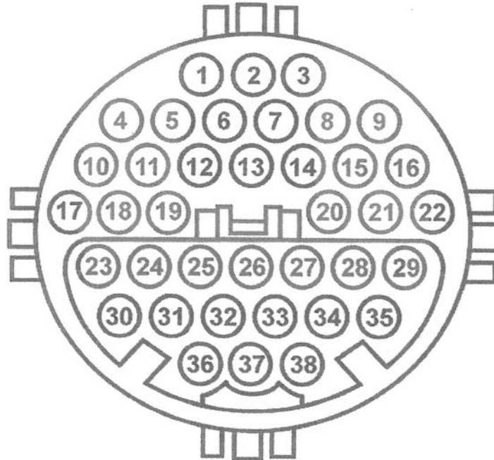
Figure 2-14. 38-pin connector—fits MB-1 adapter
