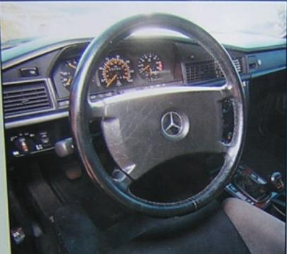
Rocker switch just right of headlight switch controls ride height; each car's series number (this one is 250) appears atop shift knob.
