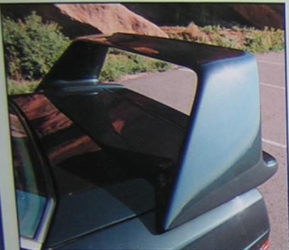
Rear wing, attached to trunk lid, extends rearward and over fenders; top element is adjustable.
