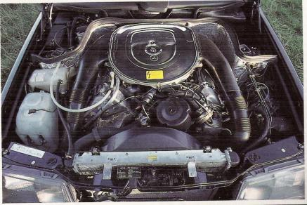
Thrust from 360bhp 32valve 5.6litre Merc V8 ensures AMG auto saloon will out-accelerate Countach from 60-120mph. Top speed is
