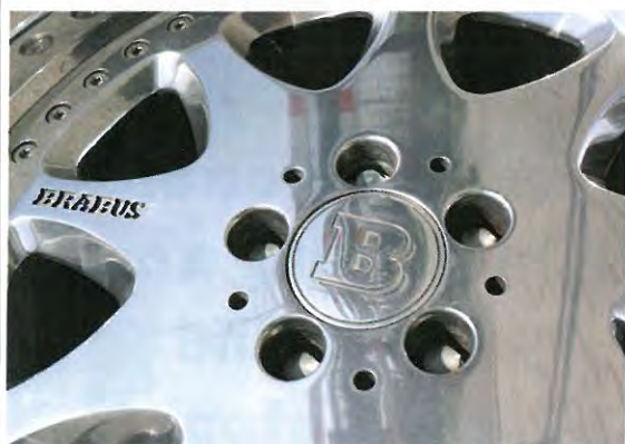
△ Three-part, split rim, 20-inch Brabus wheels were fitted without modifying the body.
