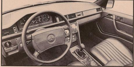
compartment is spacious and practical. The two front occupants are treated to bucket seats that offer excellent support, usefully shaped side bolsters, and a full range of power adjustment by means of Mercedes' door-mounted seat controls. These best-in-the-industry controls are supplemented by electrical adjustments for headrest height and steering-column extension. In addition, two sets of driver's seat and steering-wheel adjustments can be stored in and recalled from a memory.
