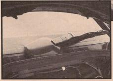
Mercedes' single windshield-wiper arm reduces high-speed skipping by sweeping parallel to the airflow. The wiper's pendulumlike base houses planetary gears that extend the arm to sweep much closer to the upper corners of the glass than a single wiper normally allows.
