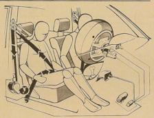
sions. In such accidents, conventional seatbelts are far more effective, and Mercedes-Benz has taken a major step to make them even more beneficial: the same sensor that triggers the air bag also activates a small powder charge that removes the slack from both front belts by turning their takeup reels. This tightening lessens both the chance that injuries will be suffered and the severity of those that do occur.
