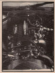
tion chambers for optimum combustion and a naturally high resistance to detonation. Mercedes has made the most of this advantage with a high compression ratio of 9.7:1, although premium fuel is recommended.
