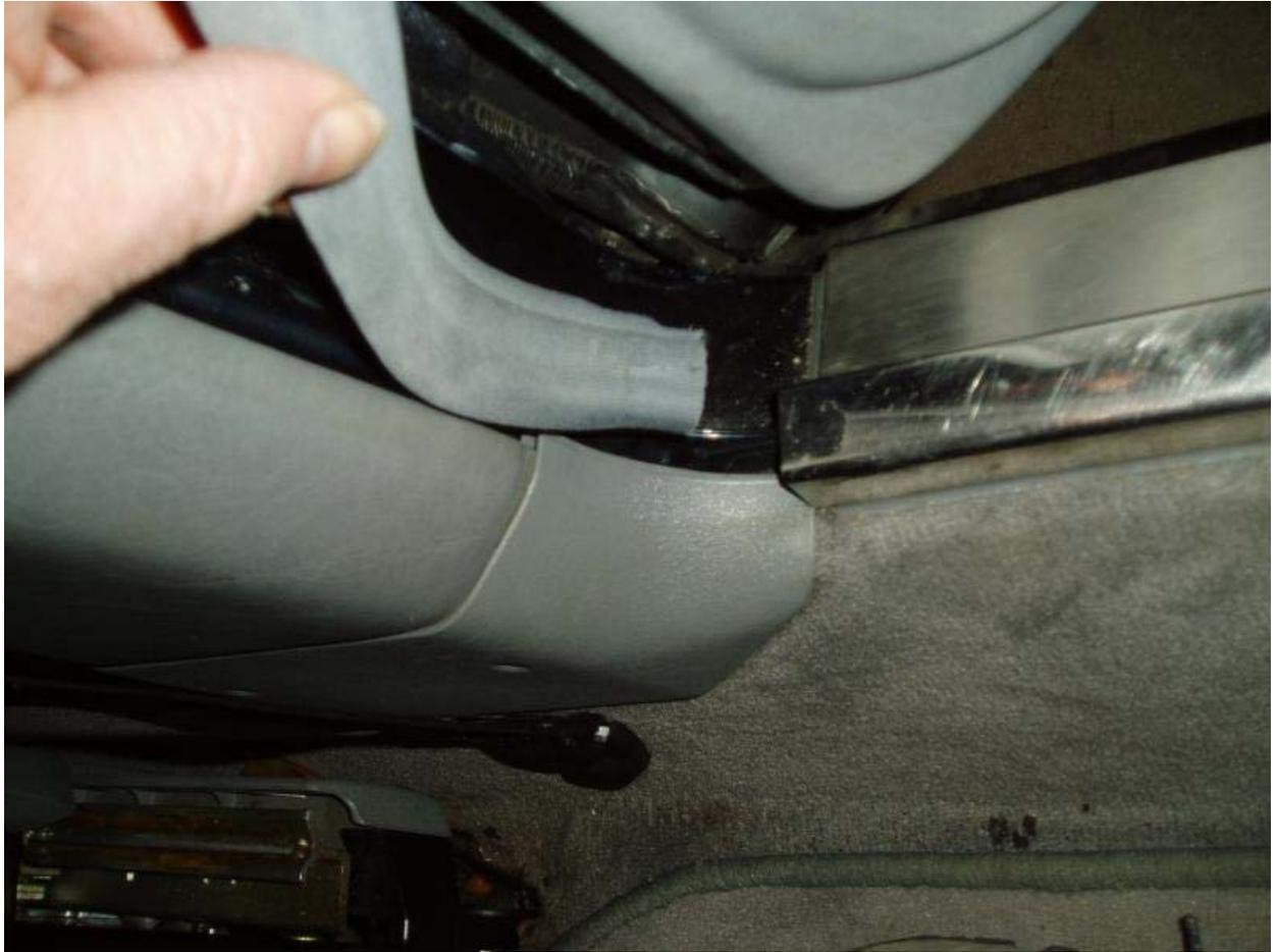
The header panel is almost free. Check along the windshield / front of the panel for urethane sealant. Sometimes when the glass is replaced some sloppy application of sealant will glue the panel to the glass. This will have to be cut free with a razor blade along the glass or equivalent.
