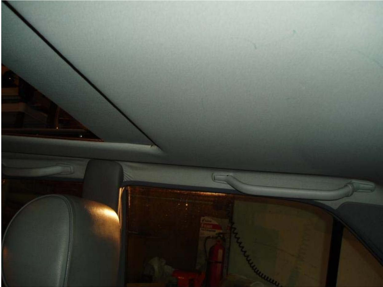
Installation is pretty much the reverse of the above. I did it in this order: sunroof opening rear, rear light & bracket, rear passenger assist handles, C-pillar panels, B-pillar panels (be careful to line up the seatbelt height adjuster handles) rear-door seals, move seats back, front assist handles, sunroof sides, header panel & end clips, header accessories, front door trim, sunroof trim.
