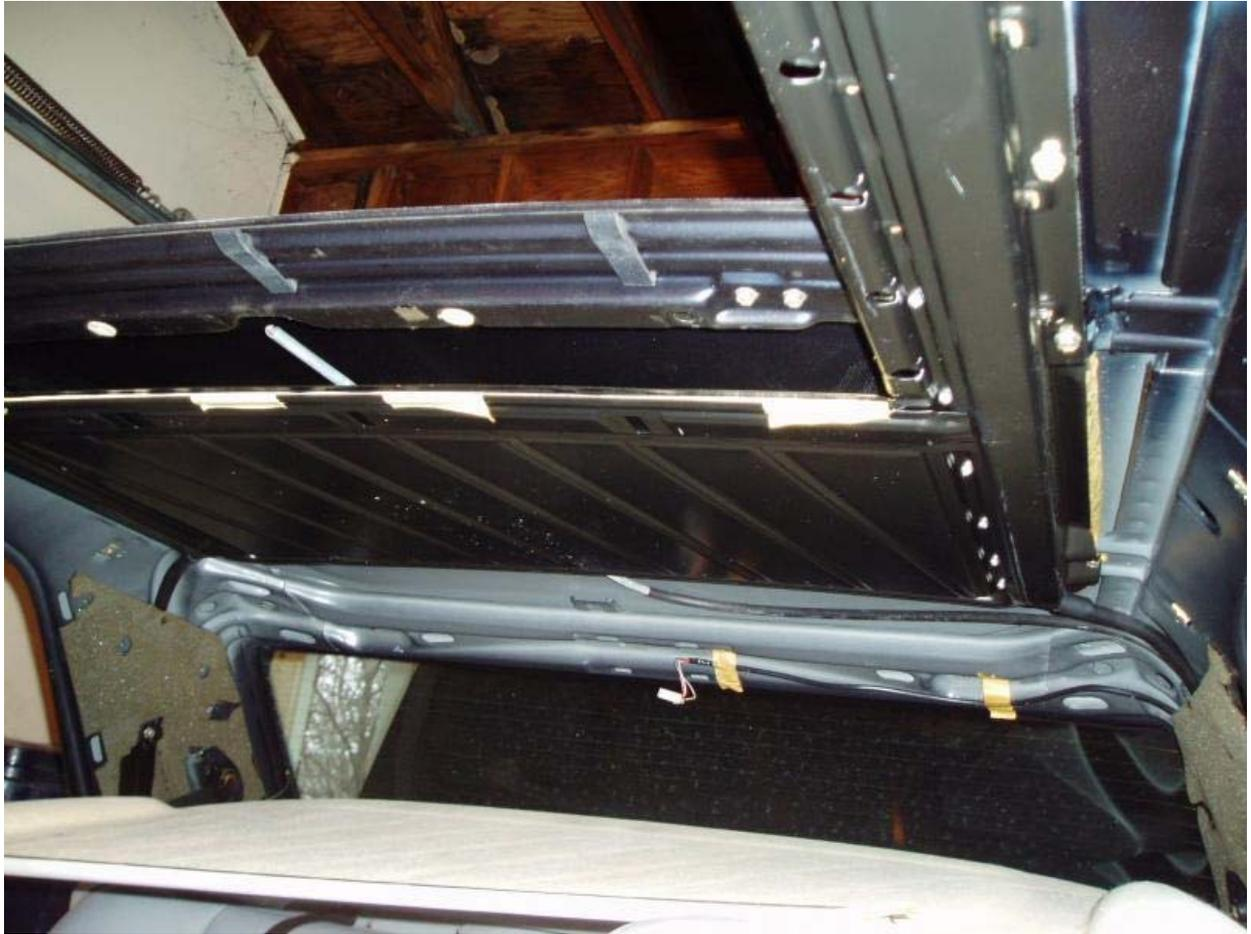
Here are a couple of photos of the removed headliner from the top (pics 1&2). Note the part number (for the gray/grau) and the aforementioned aluminum clip at the rear of the sunroof opening:
