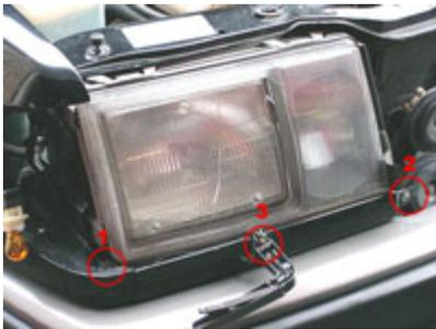
If your car has headlight wipers/washers fold down the wiper arms, undo the 8 mm nut(3) and wiggle the arms off the shafts.
