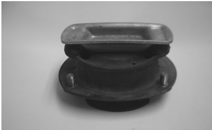
MB Stock Shock Tower MB PN: 1243200473 (124.230 and 124.290) MB PN: 1243201444 (All other 124 body) MB PN: 2013200744 (201 Body Old Number) MB PN: 2013230867 (201 Body New Number)
