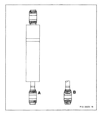
Pressed-on rubber bearing Vulcanized rubber bearing
