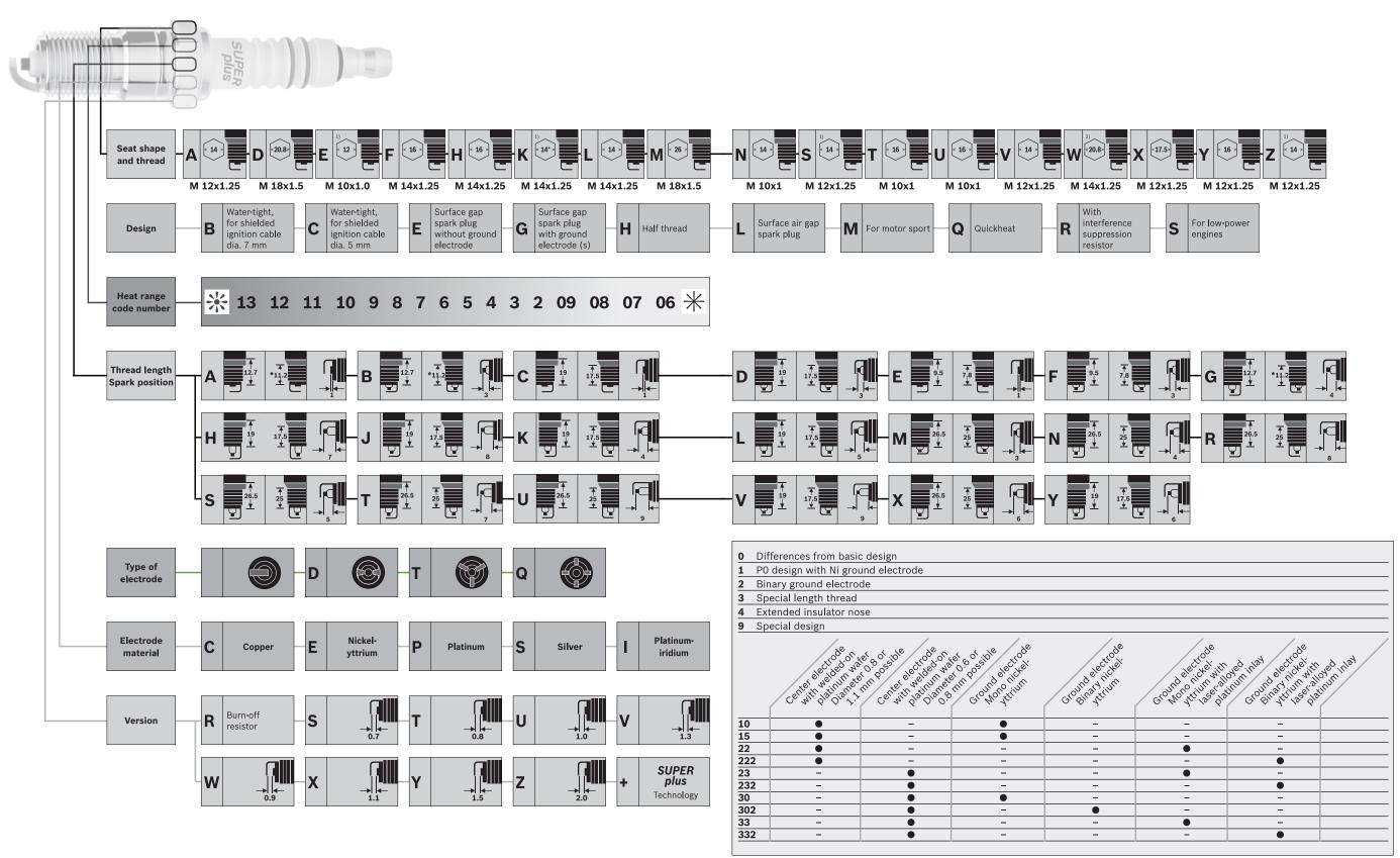
\* The thread length for spark plugs with seat shape D and spark position A or B is 10.9 mm.
