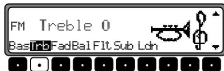
To adjust the treble, press the **SOUND** button. Then press the **Trb** multifunction key and adjust the treble to the desired level by turning the right knob
