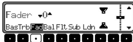
To adjust the fader between speakers, press the **SOUND** button. Then press the **Fad** multifunction key and adjust the fader setting to the desired level by turning the right knob
