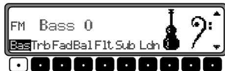
To adjust the bass, press the **SOUND** button. Adjust the bass to the desired level by turning the right knob
