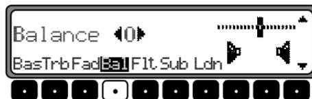
To adjust the balance between speakers, press the **SOUND** button. Then press the **Bal** multifunction key and adjust the balance to the desired level by turning the right knob
