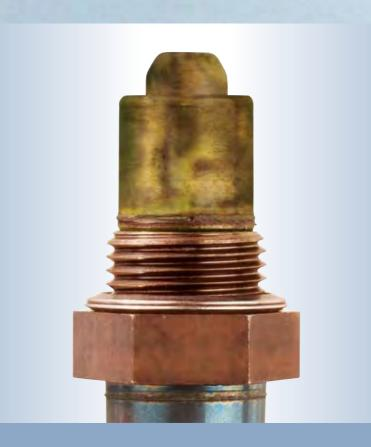
**State of oxygen sensor:** Greenish, grainy discoloration
