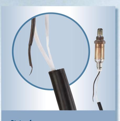
**State of oxygen sensor:** Broken cable
