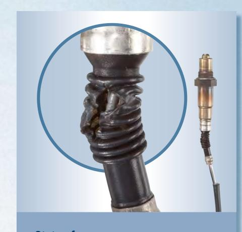
**State of oxygen sensor:** The molded cable tubing is damaged.
