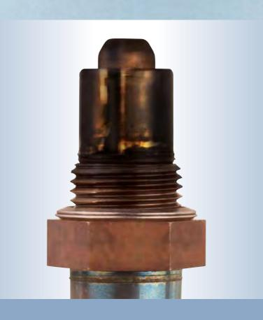
**State of oxygen sensor:** Blackened, with oily contamination
