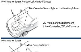
V6 or V8, Transverse Mount 1 Pre-Converter, 1 Post-Converter
