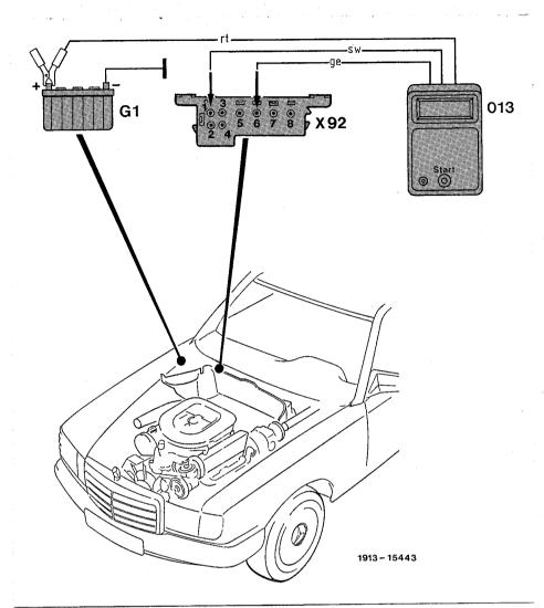
013 Pulse meter G1 **Battery** X92 Test coupling for diagnosis, 8-pin, flashing code
