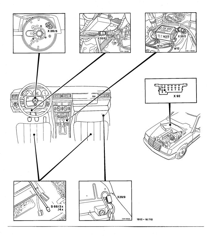
S68/3x Plug connection, belt buckle switch, airbag/belt
