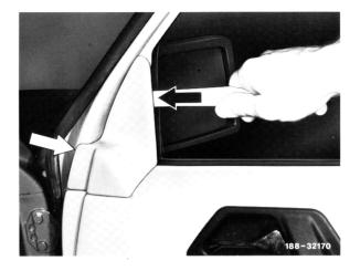
2 Unscrew fastening screw on electric plug connection and pull off plug (electric motor and mirror glass heater).
