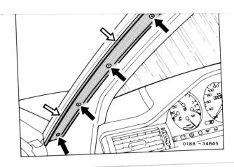
4 Insert sheet metal clip into holding rail (bore at level of rear edge of crank window).
