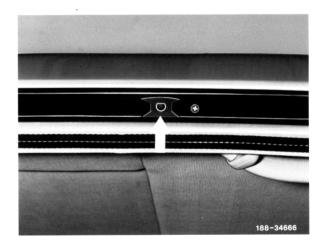
5 Position sectional sealing strip with contact surface against center of sheet metal clip, then push in sealing profile strip first toward the rear, then forward into holding rail using plastic wedge for this purpose.
