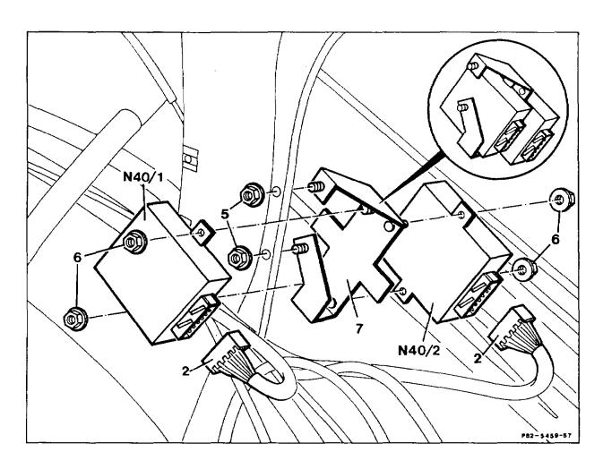
Coupling with locking bar (2) ...... release and take off, plug in and lock.
