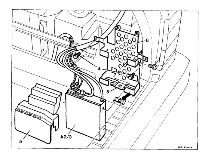
Ground cable at battery ...... disconnect, connect. Right side trim panel ...... open, close. take off, insert. Bolts (4) ...... unscrew, screw in. Electrical connections, antenna, data and speaker wiring ...... unplug, plug in. Receiver and amplifier (A2/3) with bracket . . . . . . remove, insert. unscrew, screw in. Receiver and amplifier (A2/3) ..... remove from bracket (6), insert.
