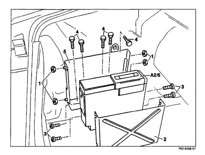
Battery ground cable ..... disconnect, reconnect. screw off, screw on. remove, install. screw out, screw in. CD player with changer (A2/6) ..... remove, install. Electrical connections on CD player with changer (A2/6) ..... disconnect, reconnect. Screws (4) ..... screw out, screw in. remove, install.
