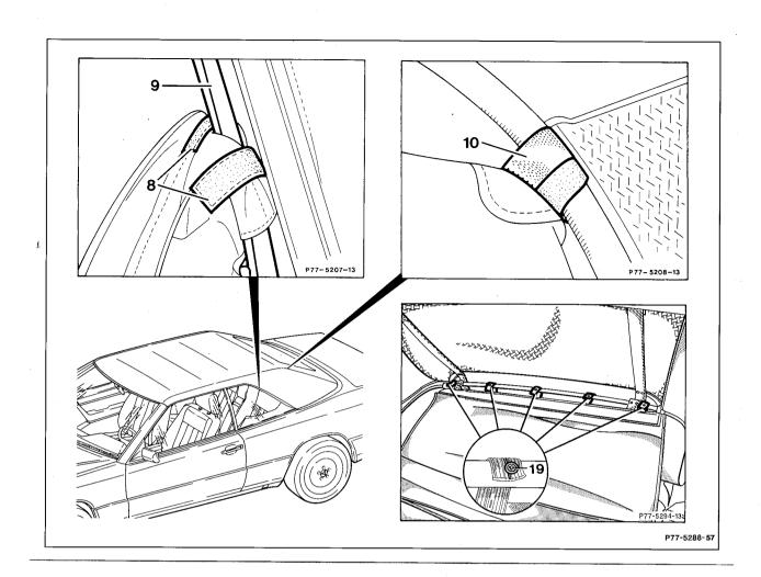
Velcro strip (8) on main pillar (9)open, close (item 71).Velcro strip (10) on corner braceopen, close (item 70).Screw (19)screw out, screw in (item 13).Intermediate layerdetach from braces, glue on (items 66–67).
