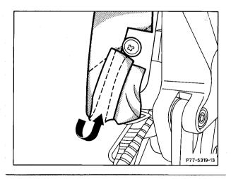
53 Press cover strip onto soft top bow and cut off with scissors.
