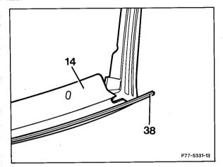
85 Glue protruding bottom strip (38) onto soft top frame folded inward (arrow).
