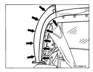
37 Fasten rubber strap (25) on soft top bow and cut off along marking.
