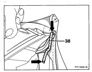
86 Install rail (15) on side of soft top and press in gasket.
