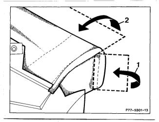
30 Fasten cover to outside of soft top frame with clips 124 589 02 37.
