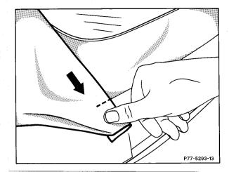
50 Pull out rubber strap (33), put up soft top bow, position cover strip with chalk mark on soft top bow (arrows, fold cover strip around and have second mechanic drill 2.5 mm dia. hole).
