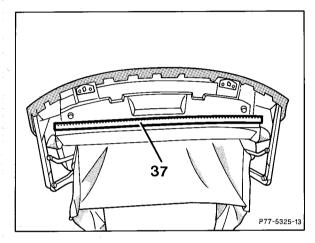
68 Press rail (7) onto braces, screw in screw (18) and hook headlining onto soft top frame. Press hooks on attachment strip together slightly.
