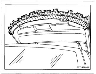
27 Pull cover down at front and position on soft top frame with marking (arrows).
