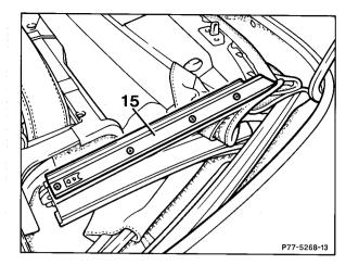
65 Glue cover strips (29) onto braces and soft top frame.
