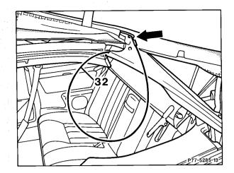
16 Rivet cable (32) to soft top frame.
