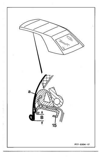
Dimension "B" = 10 -2 mm a = Cover 15 = Rail 66 Apply glue to braces, hook intermediate layer (36) onto soft top frame and glue onto braces (arrows). Press hooks on attachment strip together slightly.
