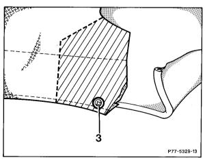
82 Press MB sealing cord 001 987 56 46 (arrows) onto cover strips (1, 2).
