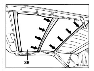
67 Glue foam rubber strips (37, 2 each) on top of one another at front of attachment strip.
