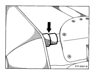
8 Check felt (arrow) on front brace, replace, if required.
