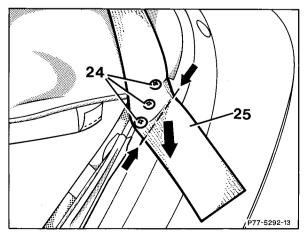
38 Open soft top at front, press soft top frame up, put up soft top bow, open soft top compartment cover and put soft top bow back down.
