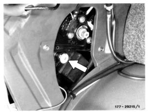
7 If the sun roof does not close accurately with this basic adjustment, move adjusting knob again into adjusting position and perform precision adjustment by turning knob:
