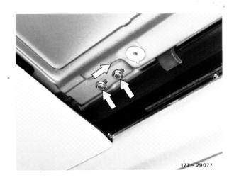
3 Since the tilting/sliding sun roof frame has tolerances with regard to its total width, the lateral clearance must be checked at several points. For this purpose, unsrew control cable on sliding carrier and move tilting/sliding sun roof top panel manually.
