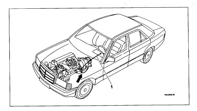
Speedometer shaft (1) at holder (arrow) ..... unclip, clip in.
