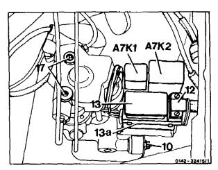
Ignition ..... Hexagon socket bolt (Torx) (8) ..... unscrew, remove plastic cover. Solenoid-valve relay (A7K1) ..... remove, reinstall. Return/charge pump relay (A7k2) ..... remove, reinstall.
