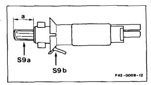
press, turn 2-pin stop lamp switch (S9) and pull out.
