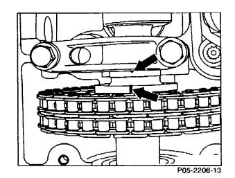
b) Inspect all the teeth of the camshaft sprocket for signs of wear. Crank the engine twice at the crankshaft for this purpose. Specified condition arrow B. If teeth tips are broken off (arrow C), or wear at tooth flanks (arrow A), replace camshaft sprocket and timing device.
