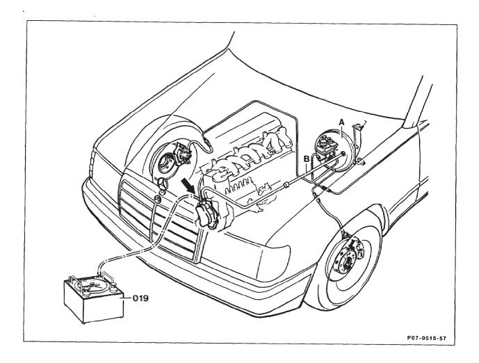
disconnect at brake booster (A). detach, and use 0.8 mm gauge to check that restriction orifice is clear. Vacuum tester (019) 201 589 13 21 00 ......
