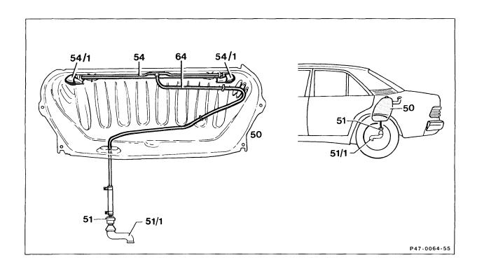
The vent system in the fuel tank (50) consists of a central pipe (54) each with a siphon breaker (54/1) at the ends. The siphon breakers prevent fuel escaping through the vent line.
