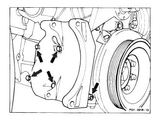
3 Unbolt return line (326) at the crankcase and withdraw from the coolant pump housing.
