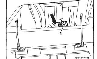
1 Drain plug on models with air conditioning
