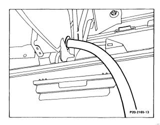
Extension hose fitted on (with air conditioning)
