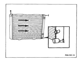
Drain plug on models with air conditioning
