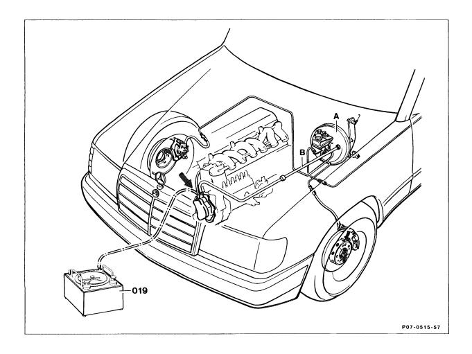
Main vacuum line (B) ..... disc Vacuum line at ancillaries connection ..... deta
