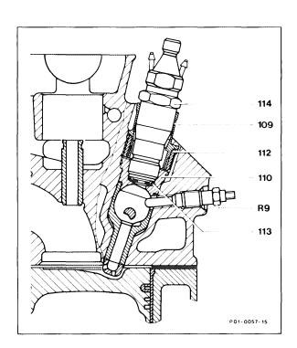
R9 Glow plug 109 Sealing sleeve 110 Prechamber 112 Threaded ring 113 Nozzle plate
