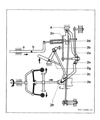
At a certain engine speed (approx. 600/min) the guide lever (2a) contacts the adjusting nut of the idle speed auxiliary spring (2o). The movement of the sliding sleeve (2h) is transferred to the injection pump control rod in the same direction via the reverse-transfer lever (2c) and the control lever (2d). After passing through the idle speed stage the sliding sleeve (2h) contacts the spring capsule (2e).
