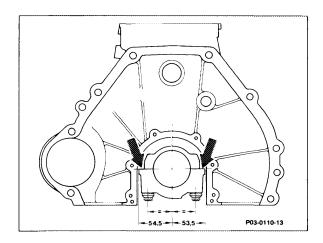
2 Lubricate crankshaft bearing bolts for crankshaft bearing caps and tighten.
