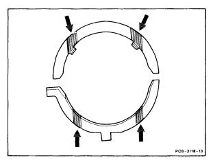
10 Position crankshaft bearing caps in proper order.
