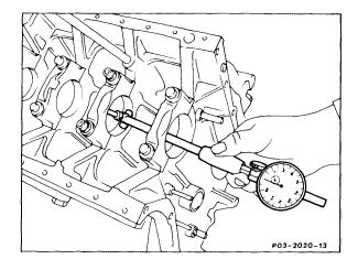
6 Measure crankshaft bearing journals, determine crankshaft bearing radial clearance.
