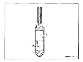
The thrust washers (148 and 148a) installed in the crankcase and in the bearing caps have a different shape.
