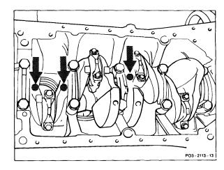
11 Tighten crankshaft bearing caps.
