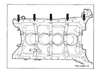
Punch marks for matching crankshaft bearing shells
