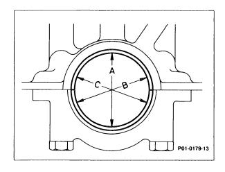
4 Remove crankshaft bearing bolts, insert crankshaft bearing shells, install crankshaft bearing caps and tighten.
