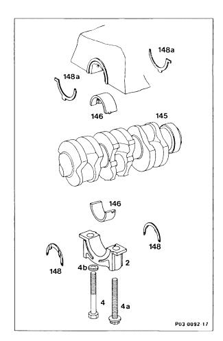
Thrust washers of the same thickness must always be installed on both sides.
