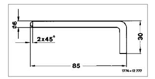
7 Plug centering pin into centering bore at left and right.
