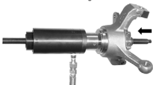
New wheel bearing insertion
