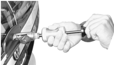
Wiper arm removal with the Slide Hammer.
