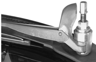
Wiper arm removal with the Pressure Spindle.
