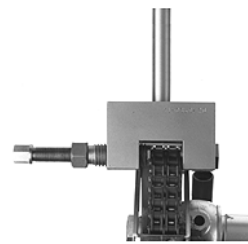
Opening of the timing chain
