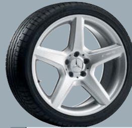
19 STYLE III AMG spoke wheel 8.5 J x 19 ET 25 · FA 255/35 R19 B6 603 1230 Sterling silver finish; only approved in conjunction with AIRMATIC DC (Code 489)
