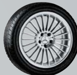
19 STYLE V AMG multi-spoke wheel 8.5 J x 19 ET 43 · 255/40 R19 B6 603 1117 Silver finish, high-sheen
