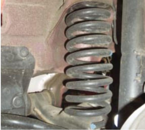
Certain models, beginning with the 140, use a small control arm at the top of the damper strut to better optimize caster and camber in certain driving modes. Some experienced mechanics find the angle of that small control arm is the quickest indication of any problem with suspension height, such as sagging springs. It pivots back as well as up in its normal travel, so once you've seen a few 'known-good's' one that's out of adjustment will leap out at you.
