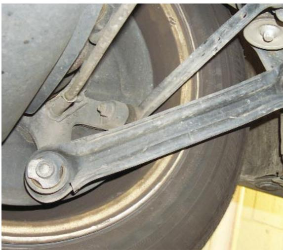
Running forward from the lowest part of the knuckle to the subframe, the pushing link transmits the drive forces from the knuckle forward to the body of the car. When the driver accelerates, the final, delivered engine torque applies to the vehicle mostly through the pushing link.
