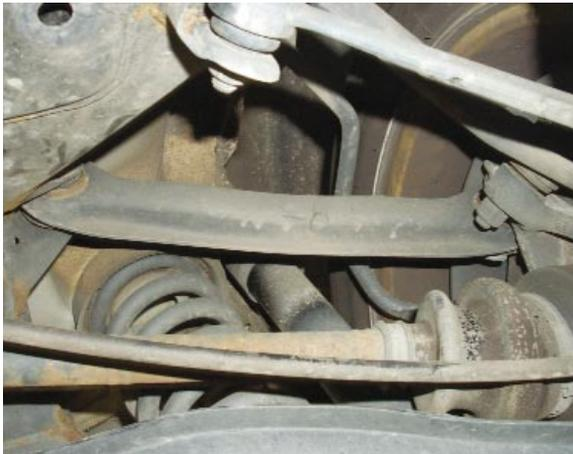
Directly above the drive axle and the spring link is the camber link, connecting the upper part of the subframe to the upper part of the knuckle. Its function is to keep the tire vertical with respect to the pavement as the vehicle corners or leans.
