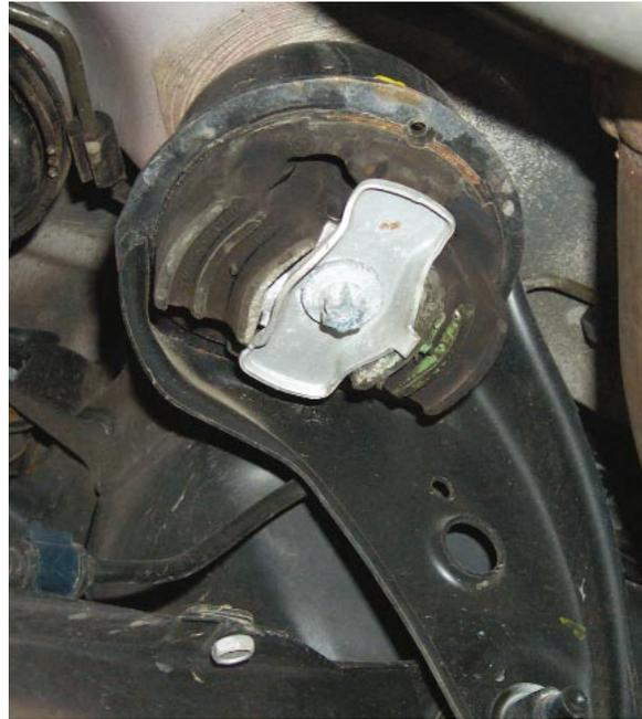
The rear suspension shares the same indirect connection to the body through a bushed subframe. The rear subframe supports the body, but it also supports the differential with separate rubber bushings. The suspension links attach to the same subframe in several positions, as we'll see below.
