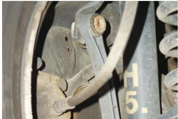
The swaybar and its bushings are above the drive axle but connect through the yoke at the outboard side of the spring link to the knuckle. Most Mercedes-Benz technical literature refers to the swaybar as a “torsion bar.” The driveshafts themselves are also, in a way, links between the differential and the wheels.
