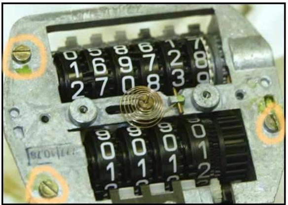
You will see the spring that controls the needle. The speedometer cable drives a gear inside, turning the pin with light friction and two magnetic rings. The faster the cable turns, the more wound up the spring gets. The spring is one of several ways the speedometer is adjusted. Unscrew the three (3) screws from the upper assembly and separate the halves.
