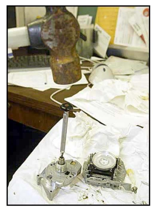
My speedometer was very stiff. I figured out the backside was knocked too far in and needed to be pulled back out. I also wanted to inspect the plastic gears while I had it apart. To do this, I knocked the drive gear out. It is held in by glue as far as I could tell.
