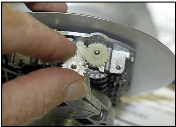
First things first. A quick fix for the gear. Simply pop off the broken gear with a screwdriver and press on the new gear. For information on new gears, go to the links above.
