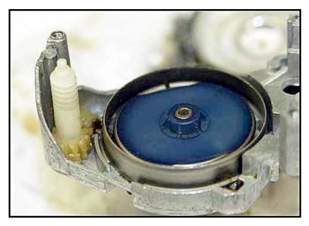
When putting the two halves back together, put the worm gear in first. Spin the drive a little until you feel the needle engage the drive gear. Put the three (3) screws back in and test spin the drive.
