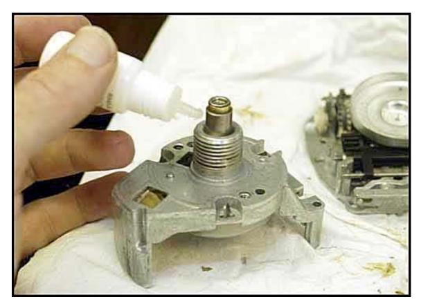
To reset the drive gear, I used common quickset glue. I carefully applied a few drops to the outside bearing and turned it in the housing until the glue gripped. Make sure you don't get any glue on the drive. The most critical part of this step is to set the drive gear to the correct height. This is why my speedometer was too stiff to begin with.
