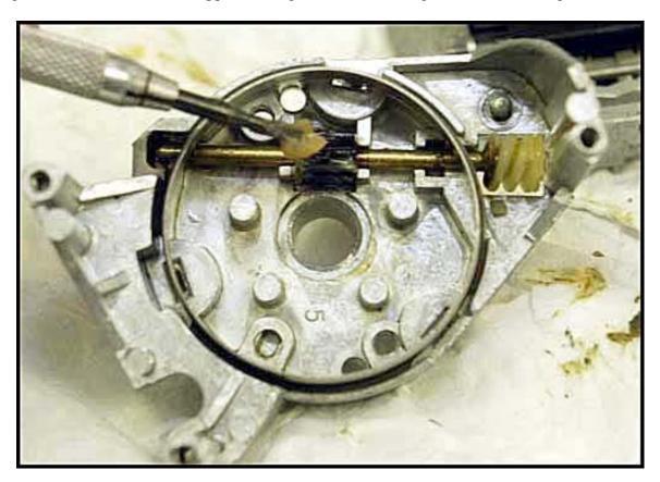
I washed out all the leftover glue and grease that worked it's way into the housing and re-applied grease to the gears. The ring holds down this shaft. If you want to remove it, use needle nose pliers to untwist the tabs. Otherwise, just use a paper towel and clean off the old grease before you re-apply the new grease.
