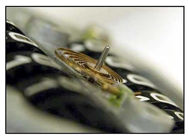
To figure out the proper position of the drive gear, when you reassemble the two halves, the needle spring should be level. If the center is low or high, the gears might not engage, the drive might be too stiff or the two halves won't fit together.
