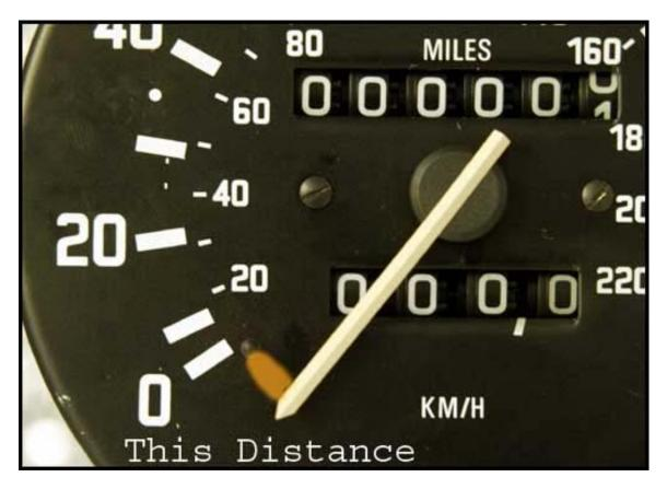
This is the part that I really am guessing about. When putting the needle back on, you need to pre-load the needle and then move it over the stop. The position of the needle in this photo was based on another speedometer that hasn't been taken apart. I would suggest a little trial and error to get the right position or stop by your local garage and get it recalibrated.
