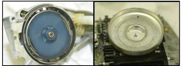
(Left) The pin from the top section fits delicately into the center of the blue section that links to the speedometer cable. As the cable turns the blue "disc", the pin also turns loosely, driving the needle. (Right) This is the bottom of the upper section. The pin is the bottom end of the needle.
