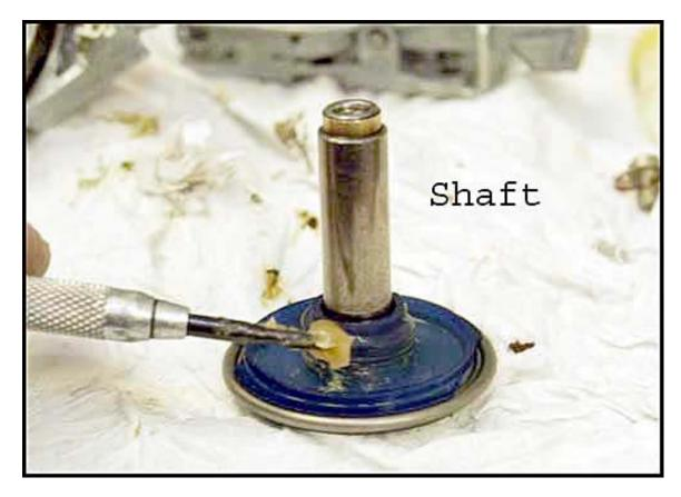
Using a small screwdriver, I re-applied axel grease to the drive gear, careful not to get it on the shaft.
