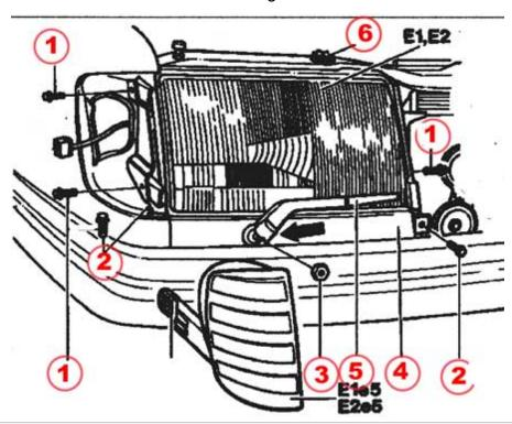
After disconnecting the battery remove the old blinkers. Look at he clip on rear of new blinker to see how it works. Behind each side blinker unplug the power socket, release the tab, and push out the assembly.
