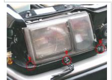
If your car has headlight wipers/washers fold down the wiper arms, undo the 8 mm nut(3) and wiggle the arms off the shafts.
