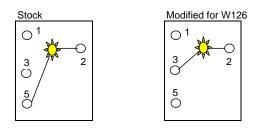
Re-solder wire from LED at terminal 5 to terminal 3, which is ground at all times
